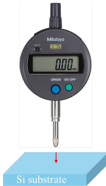
Fig. 3.2.1.1 Illustration of the measurement using the digimatic indicator [1].
